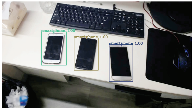
Fig. 4. Smartphone detection for RBC system. Each smartphone is marked with a bounding box and a class label.
